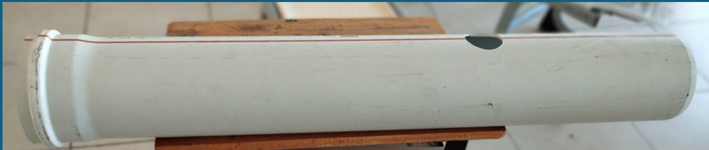
PVC pipe for telescope tube
